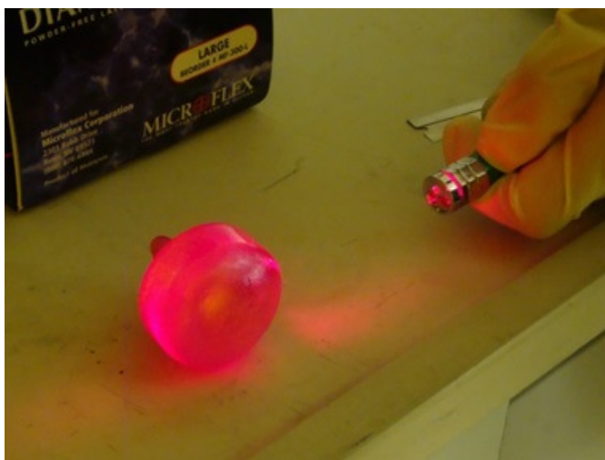
Mercurous halide imaging-quality crystals grown by physical vapor transport.
